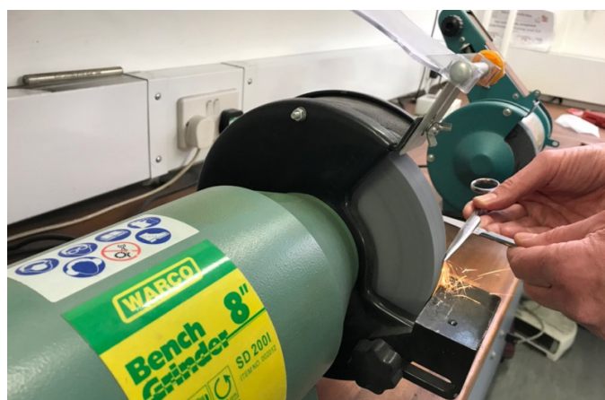
Figure 12: Repair of surgical scissors
